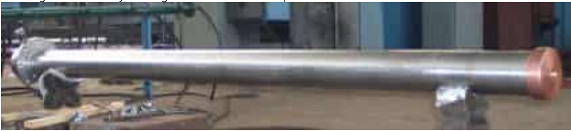
Plasma torch for titanium refining. Power up to 1 MW, dimensions: diameter 180 mm, length 3.5 m
